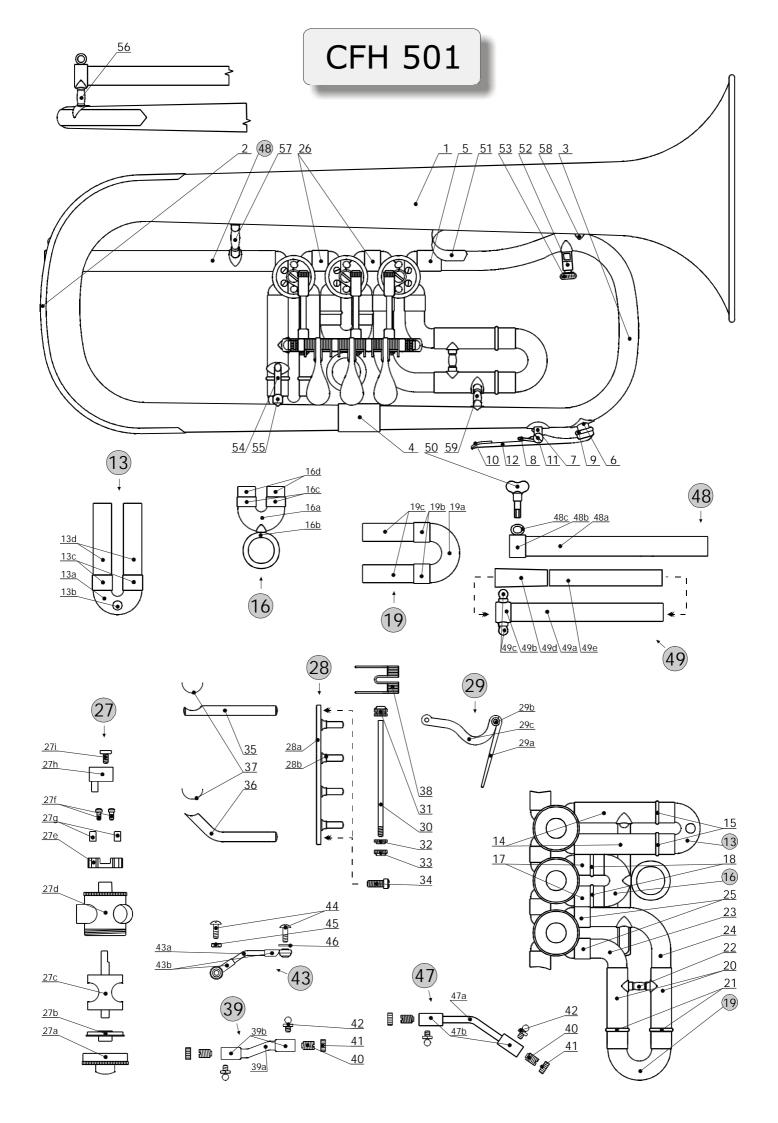
Parts For V.F.Cerveny Bb Rotary Valve Fluegelhorn CFH 501.
